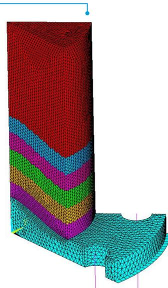
The effective elastic properties of the lattice material were associated to an equivalent homogeneous solid that replaces the lattice domain. These orthotropic properties were obtained from the structural analysis of a single representative volume element: the unit cell.
