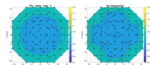
It is evident in these validations the similarity in the two stress distributions and in the Δσ values: 3.2 % for the homogeneous model and 3.4 % for the cellular model.
